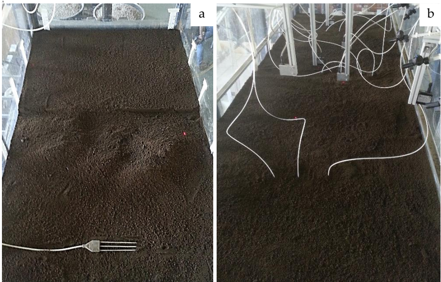
Figure 37: a) reconstruction of the deposit by layer, with the TDR probe placed in position; b) installation of the porous caps of the tensiometers.
