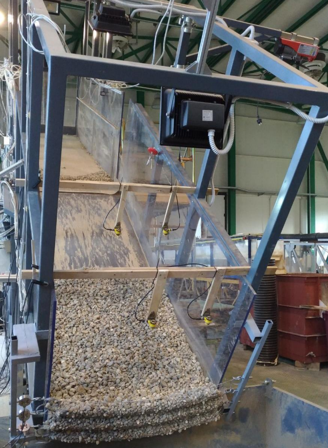
Figure 58: Test conducted in collaboration with the University of Parma: configuration of the flume at the end of the test.
