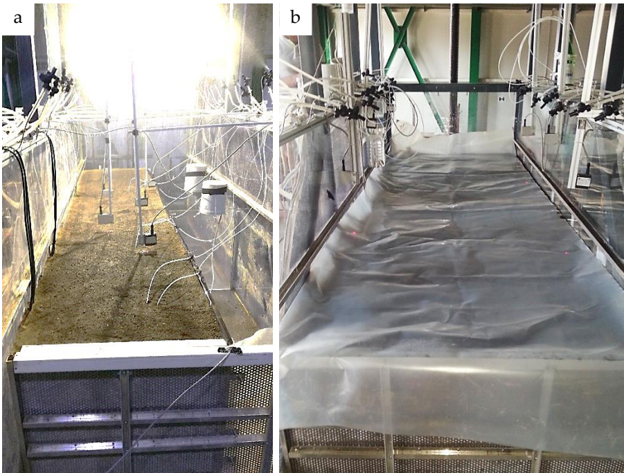
Figure 38: a) Low-intensity rainfall phase with the deposit in a horizontal position. b) Deposit covered by a plastic sheet.
