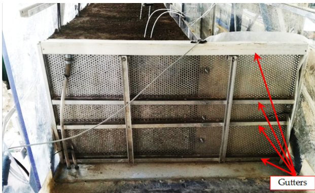
Fig. 6. View of the perforated panel, placed at the foot of the physical model of a layered slope, aimed at realizing a seepage face boundary condition, and provided with gutters (indicated with the red arrows) for the separate collection and measurement of overland and subsurface runoff coming from the three layers. (For interpretation of the references to colour in this figure legend, the reader is referred to the web version of this article.)
