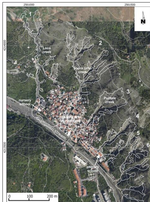
Figure 23. October 2009 debris flows occurred in GiampilieriSuperiore, obtained by interpretation of aerial photo
