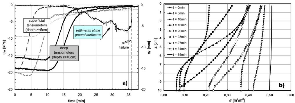
Figure 5. Records of suction and settlement of the ground surface (a) and assessment of the volumetric water content (b) in a flume test (Damiano et al., 2008)
