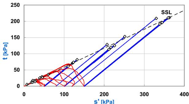
**Figure 18. Results of drained and undrained CID and CIUC tests on natural samples of Sarno volcanic ash**
