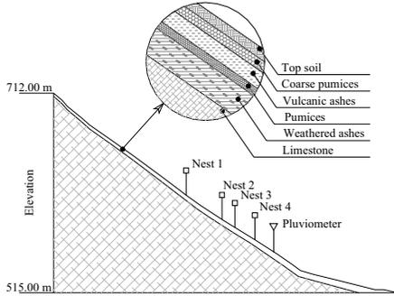
Figure 3. The instrumented Cervinara slope
