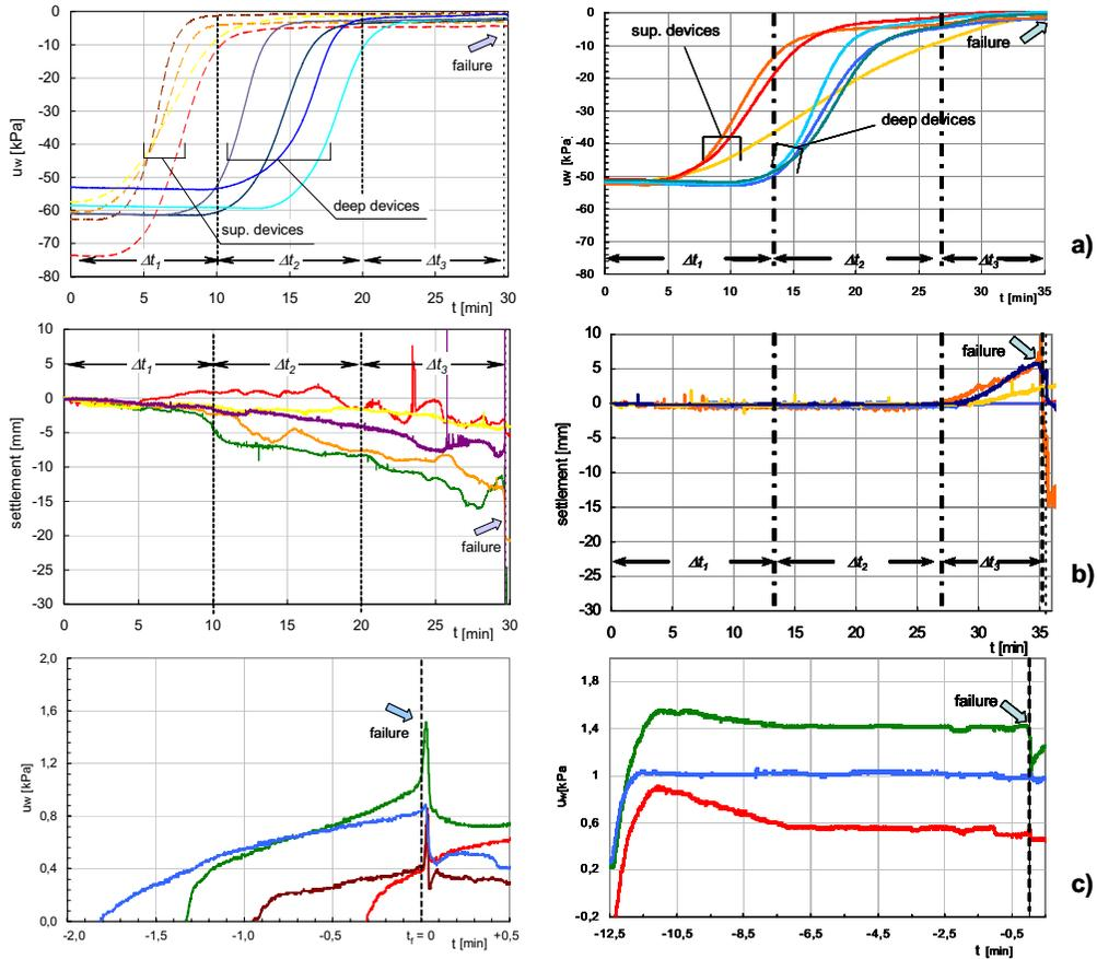
Figure 2. Results of a flume test carried out on the Cervinara volcanic ash (loose soil on the left side; dense soil on the right side): a) suction measured at two different depths; b) settlement of the ground surface; c) pore pressure recorded at the base of the layer (modified from Damiano, 2004)
