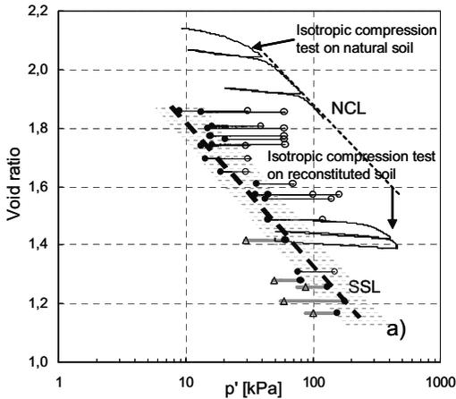
**Figure 16. Results of undrained triaxial compression tests on reconstituted specimens of Cervinara ash, reported in the compression plane (from Olivares et al. 2003)**
