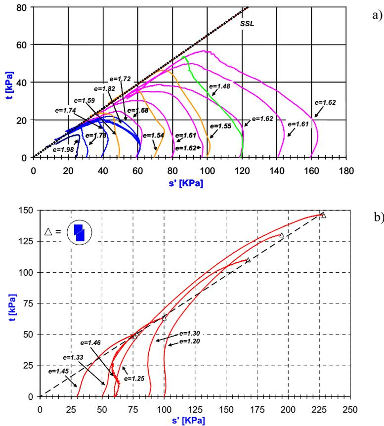
**Figure 15. Results of undrained compression triaxial tests on reconstituted specimens of the Cervinara ash (from Lampitiello 2004): a) loose specimens; b) dense specimens**
