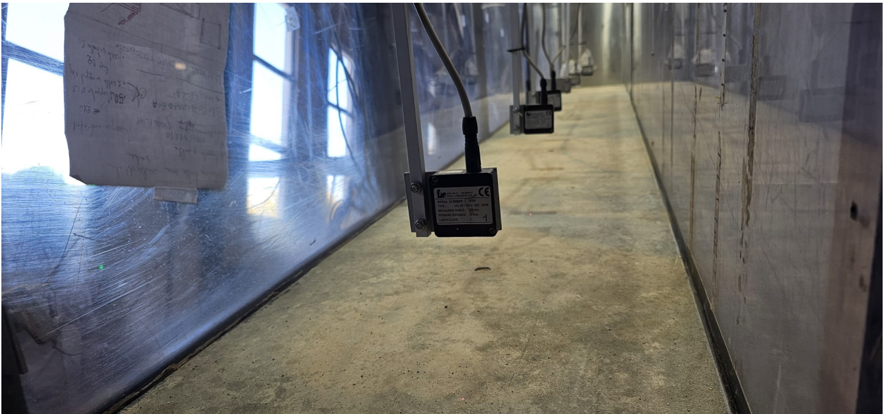
Figure 8. Detail of the laser distance meters and the rough carpet.
